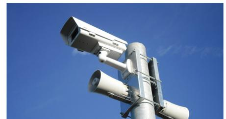
Vi-System integrated with AXIS Q1921-E Thermal Network Camera
